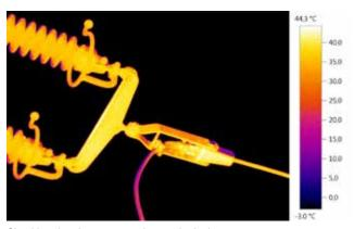
Checking the clamp connection on the isolator
