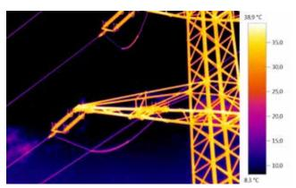
Thermal image of the current loop on a dead-end tower
